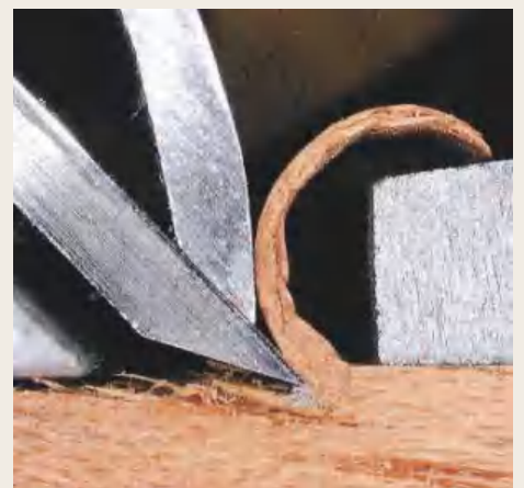
▲ Pic.4 Planing against the grain using a cap iron. Note the torn surface, the stress marks and the kinks in the shaving
